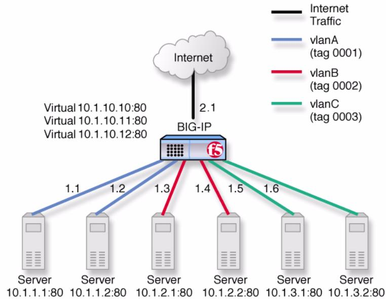
*Figure 6.2 Multiple customer hosting using VLAN switching*
