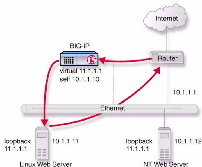
**Figure 19.1** An example nPath configuration
