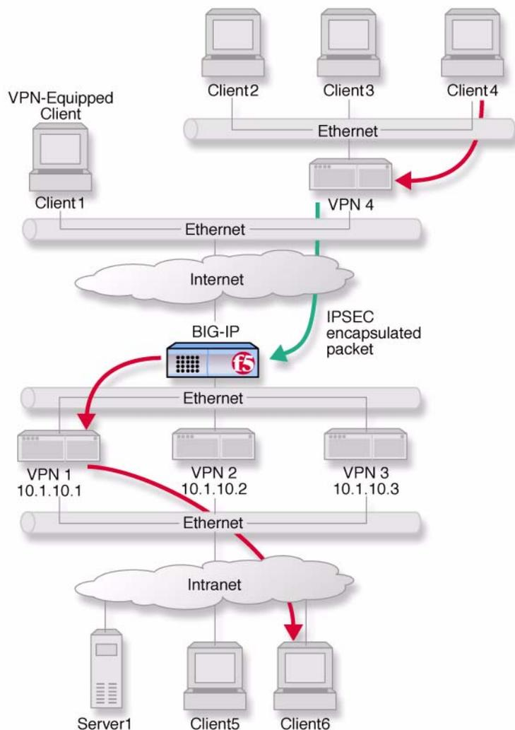
**Figure 10.1** VPN load balancing between VPN gateways
