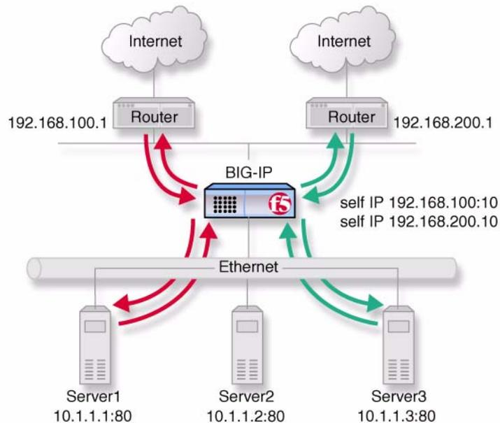
*Figure 8.1 An example of an additional internet connection*
