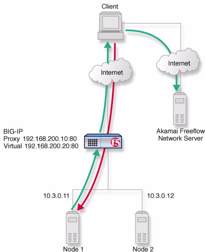
**Figure 16.1** Content converter configured on a BIG-IP system
