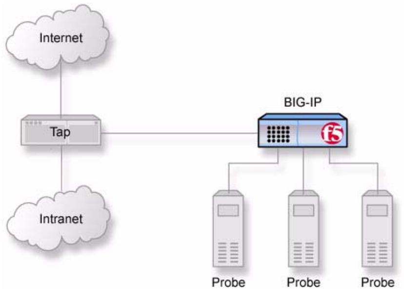
**Figure 4.2** An example out-of-band configuration with VLAN mirroring.
