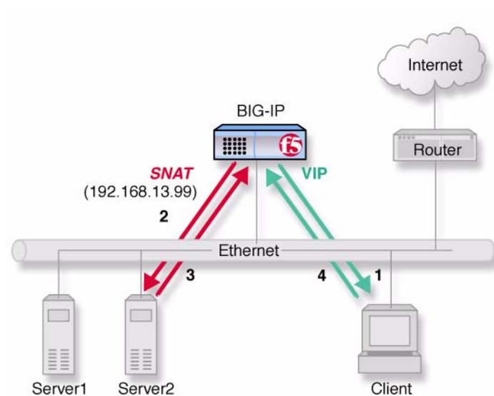
**Figure 18.1** An example of a single interface topology
