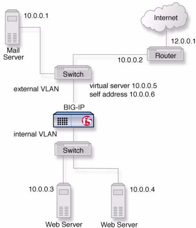
*Figure 3.2* New structure after adding the BIG-IP system
