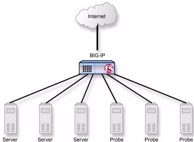
*Figure 4.6* An in-band configuration for clone pools
