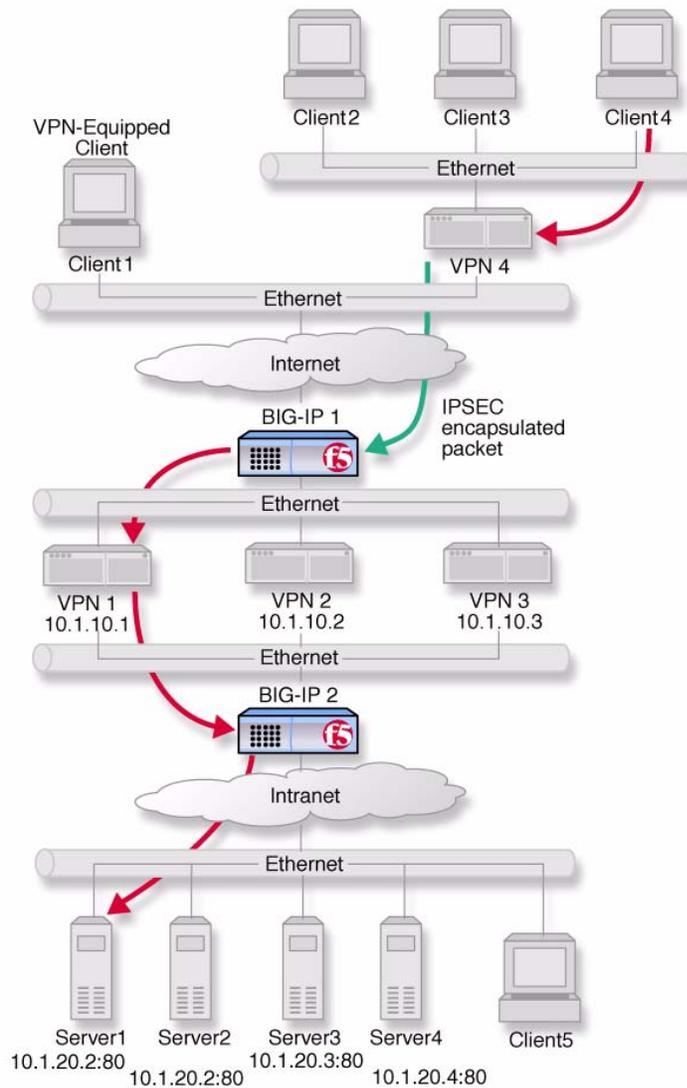
*Figure 10.2* VPN load balancing between VPN gateways
