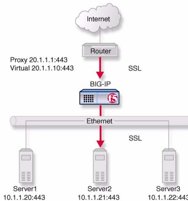
**Figure 11.5** An incoming SSL connection with SSL-to-server
