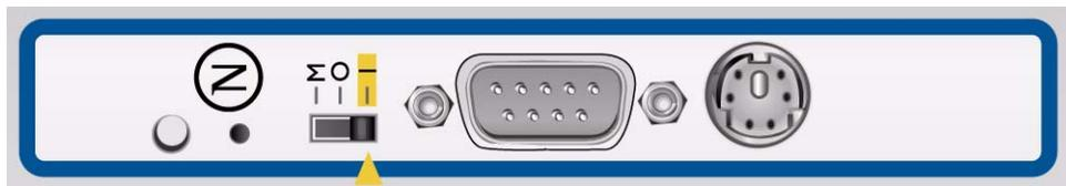
*Figure 1.1 This figure shows the M-O-I switch on the FIPS 140 security module*
