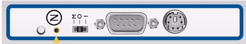
**Figure 1.2** The reset button on the FIPS 140 security module
