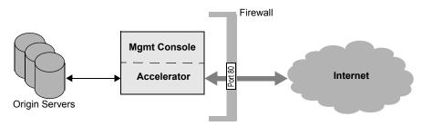
For a multi-machine WebAccelerator installation, one machine has the Management Console and an Accelerator, and the other machines each have a single Accelerator or WebAccelerator Remote:
