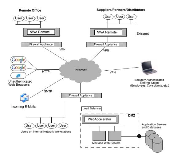
In this case, all the WebAccelerator Remotes and WebAccelerators belong to one cluster, and this cluster is assigned to both the mail server and web server applications. A cluster can be assigned to more than one application, but an application can only have one cluster assigned to it.
