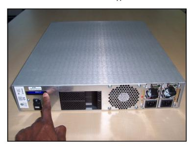
3. Insert the new CompactFlash card into the slot, and then push it in slowly until the Eject button pops up.
