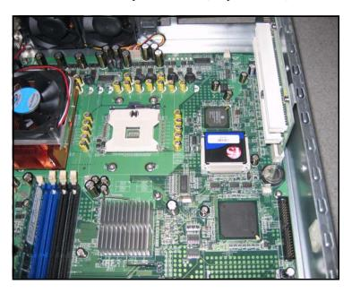
5. Remove the CompactFlash card by sliding it out of the socket toward the back of the appliance.
