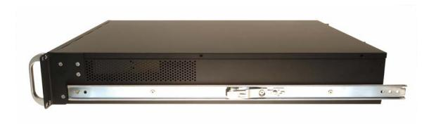
Figure A.2 An inner rail attached to the WANJet 500
