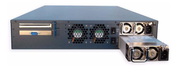
Figure 4.1 Power supply partially removed from the system
