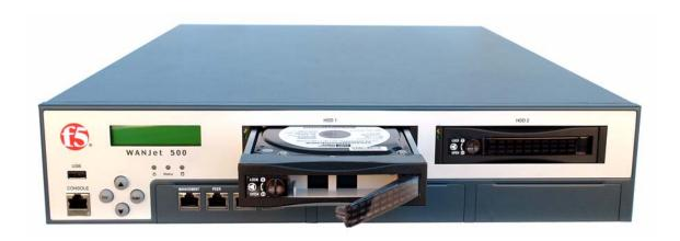
Figure 4.2 Removable drive tray and hard drive
