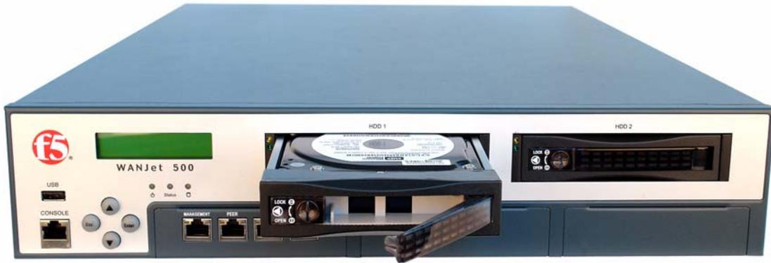
*Figure 4.2 Removable drive tray and hard drive*
