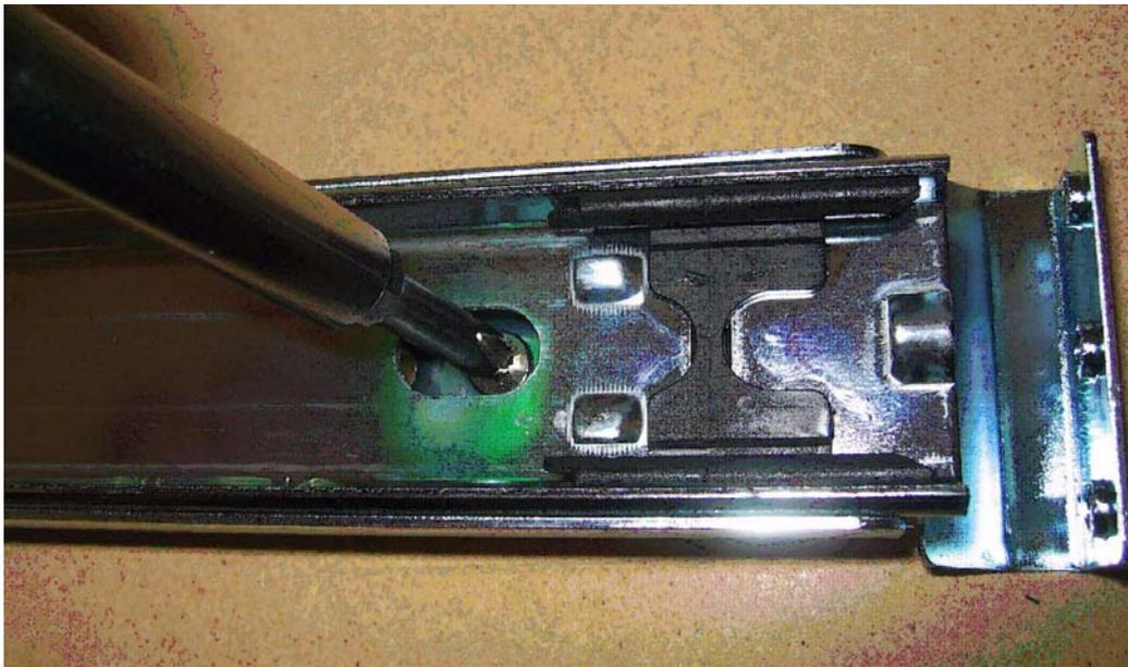
*Figure A.4 Attaching the outer rail to front of the mounting bracket*
