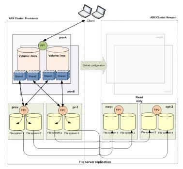
The second figure illustrates an actual disaster recovery situation, in which the Providence cluster is unable to continue operating, and the ARX administrator has executed the failover process for both the filer servers and
