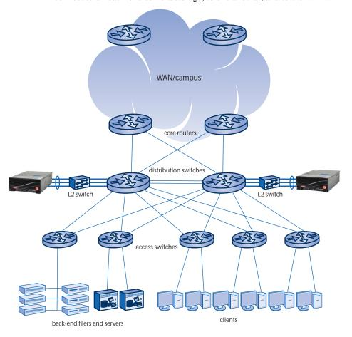
The sample network has redundant ARXes connected at each of the distribution switches. Physically, this is a one-armed connection; conceptually, the ARX has front-end clients in front of it and back-end servers and filers behind it. To simplify the examples, the access switches are removed from the remaining illustrations in the book.
