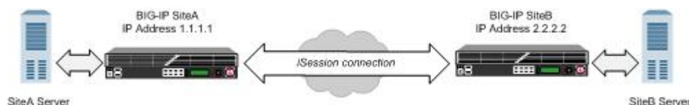
Figure 4: Network topology for a secure iSession connection
