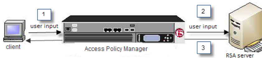
Figure 6: How Access Policy Manager works with RSA SecurID
