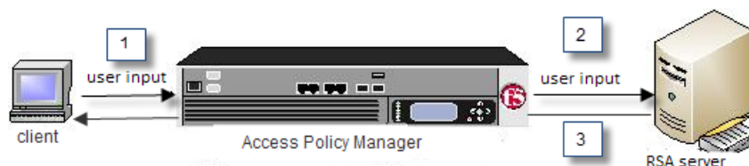
Figure 7: How Access Policy Manager works with RSA SecurID
