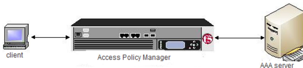
Figure 8: How RADIUS works
