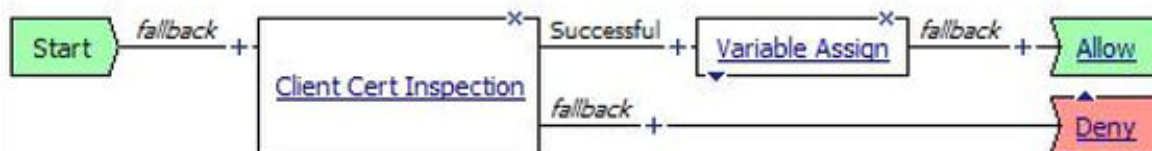
Figure 22: Example access policy for Kerberos SSO
