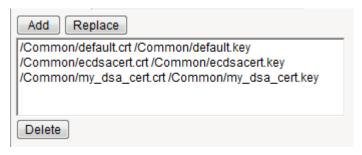
Figure 1: Sample configuration with three key types specified
