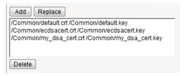
Figure 6: Sample configuration with three key types specified
