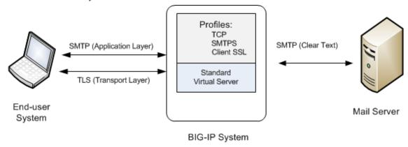
Figure 10: Sample BIG-IP configuration for SMTP traffic with STARTTLS activation
