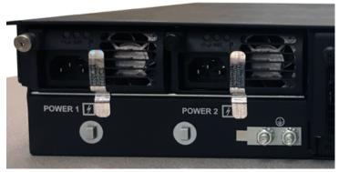
**3.** Place a tamper evidence seal so that half of the seal covers the top of the chassis enclosure and half covers the right side of the chassis, and then do the same for the left side of the chassis.
