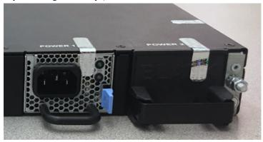
**6.** If your platform includes two externally-accessible storage drives, place a tamper evidence seal so that half of the seal covers one drive and half covers the other drive or storage drive blank.
