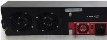
5. If your platform includes any blank covers, place a tamper evidence seal so that half of the seal covers the chassis enclosure and half covers any blank covers (for example, blanks for unused power supply bays or storage drive bays).
