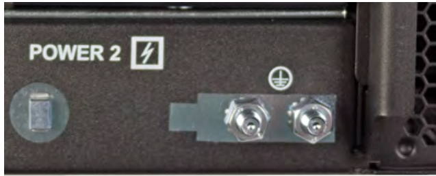
Figure 6: Chassis ground lug
