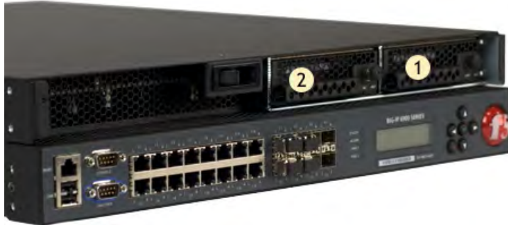
Figure 13: The front of a platform with front bezel removed and the orientation of the primary and secondary hard disk drives
