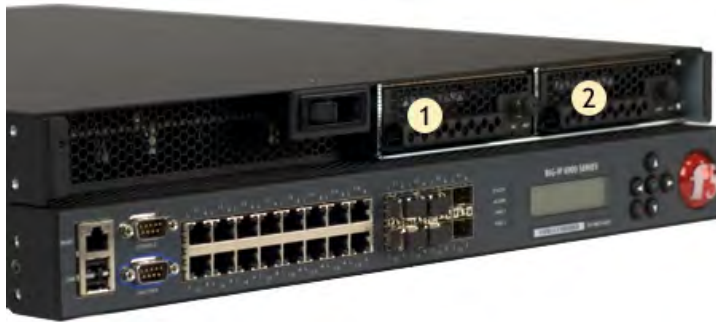
Figure 11: The front of a platform with front bezel removed and the orientation of the drive bays
