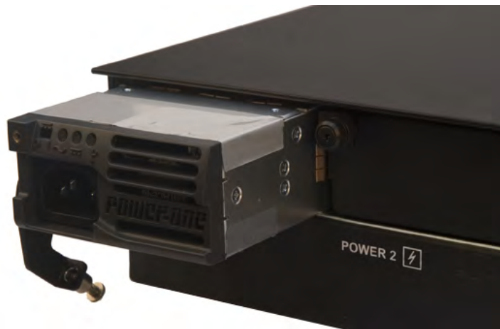
Figure 7: A power supply partially removed from the platform
