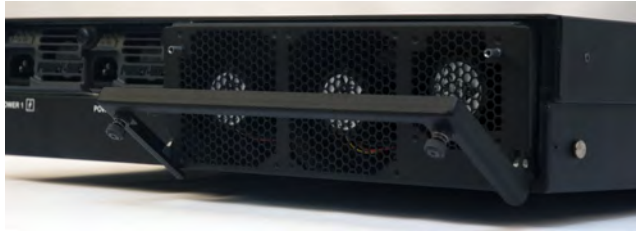
Figure 10: An example of a fan tray in a platform
