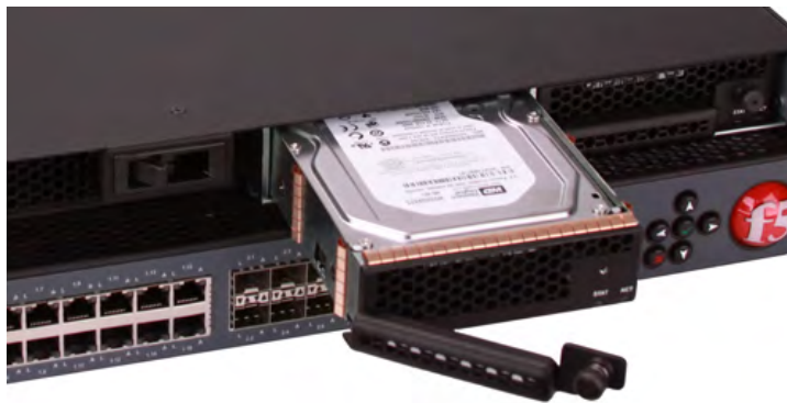
Figure 12: An example of a hard disk drive shown partially removed from the system
