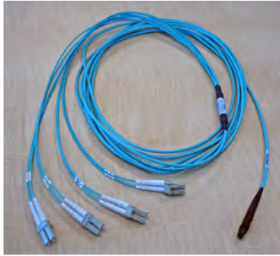
Figure 4: An example of a QSFP+ breakout cable
