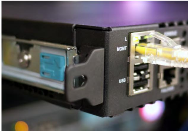
2. Slide the unit into the rack, and then secure the rail lock brackets to the rack on each side of the unit using either the two #8-32 pan head Philips screws that are included or screws provided by the rack manufacturer.
