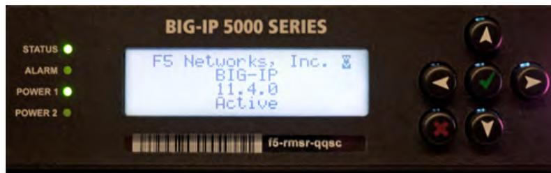
Figure 3: The LCD panel and control buttons
