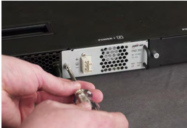
9. Connect the terminal block into the DC power supply.
