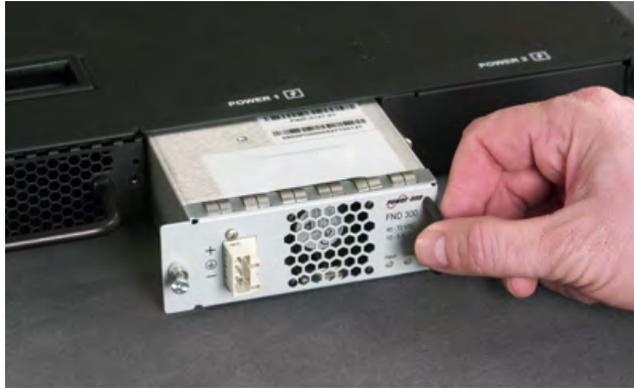
8. Tighten the screw completely, using 4 to 5 inch-pounds (0.45 to 0.56 Newton-meters) of torque on the screw.
