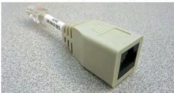
**Figure 6: The RJ45F to RJ45M rolled serial (pass-through) adapter**
