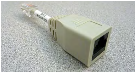
Figure 7: The RJ45F to RJ45M rolled serial (pass-through) adapter
