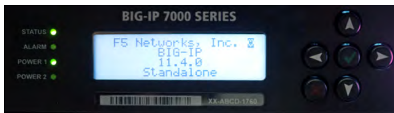
Figure 3: The LCD panel and control buttons
