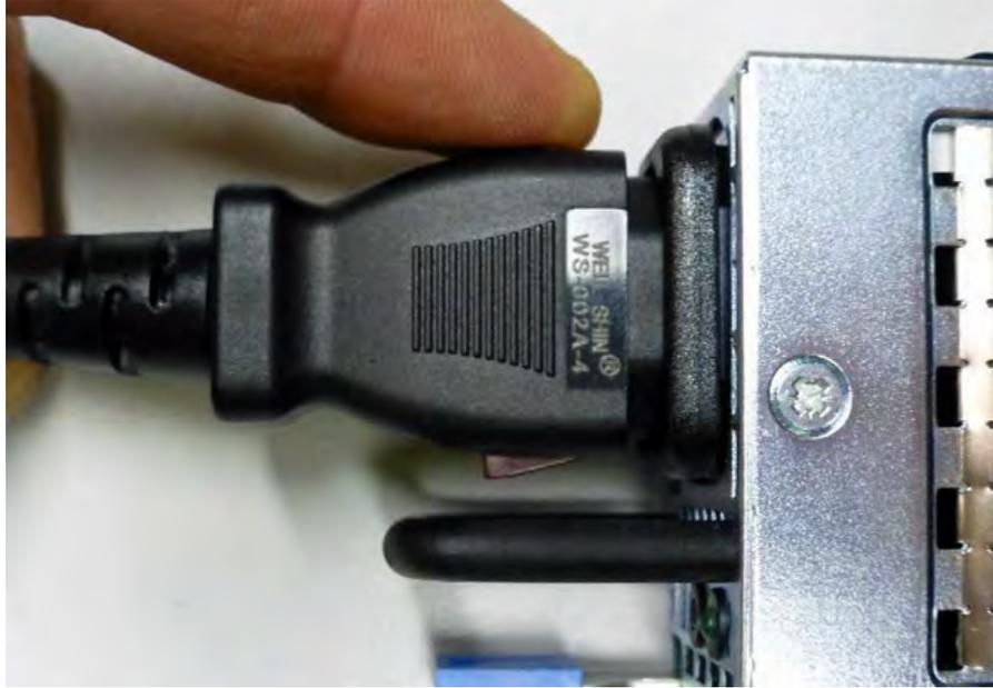
3. Remove the failed AC PSU by squeezing the ejector latch and pulling straight toward you.
