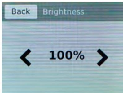
4. Use the left and right arrows to adjust the brightness of the LCD in real-time.
