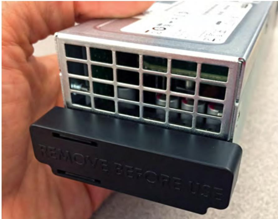
5. Inspect the new PSU, especially the connector area, for any damage that might have occurred during shipment.
