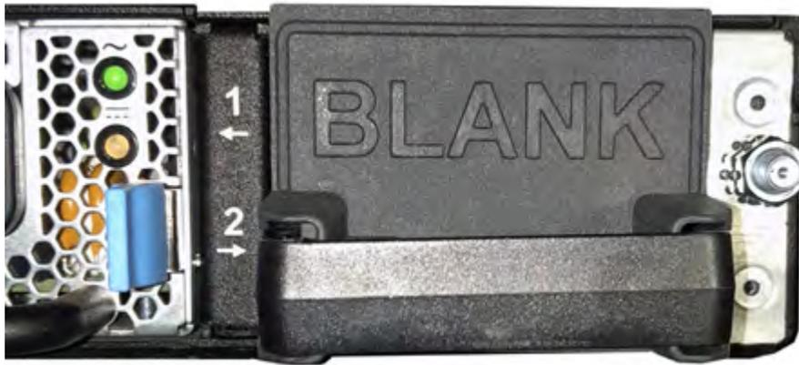
Figure 6: Chassis ground lug
