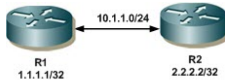
Figure 6: Basic Topology for BFD-ISIS
