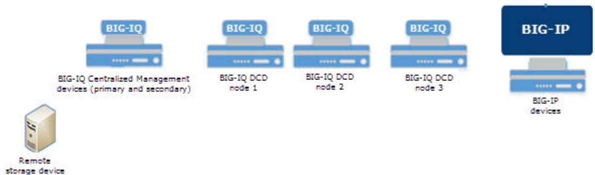
**Figure 1: Centralized Management network topology**
