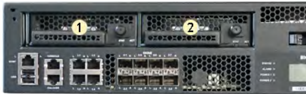
Figure 11: Orientation of the 7000 Series platform hard drive bays
