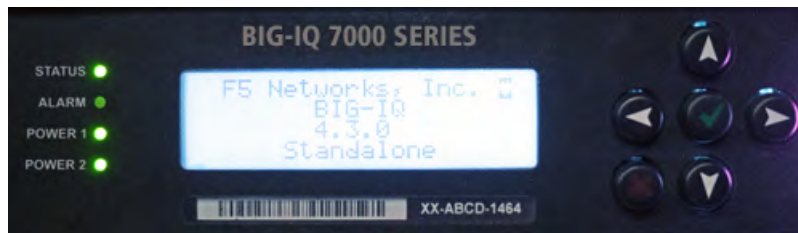
Figure 3: The LCD panel and control buttons
