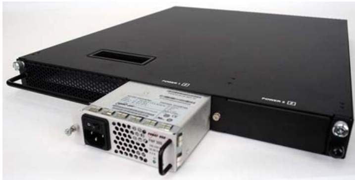
Figure 5: A power supply partially removed from the platform
