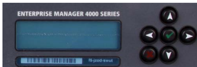
Figure 3: The LCD panel and control buttons
