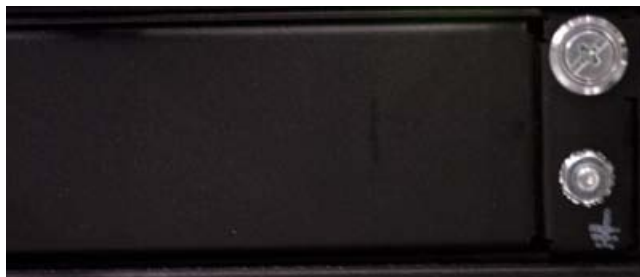
Figure 4: Chassis ground lug
