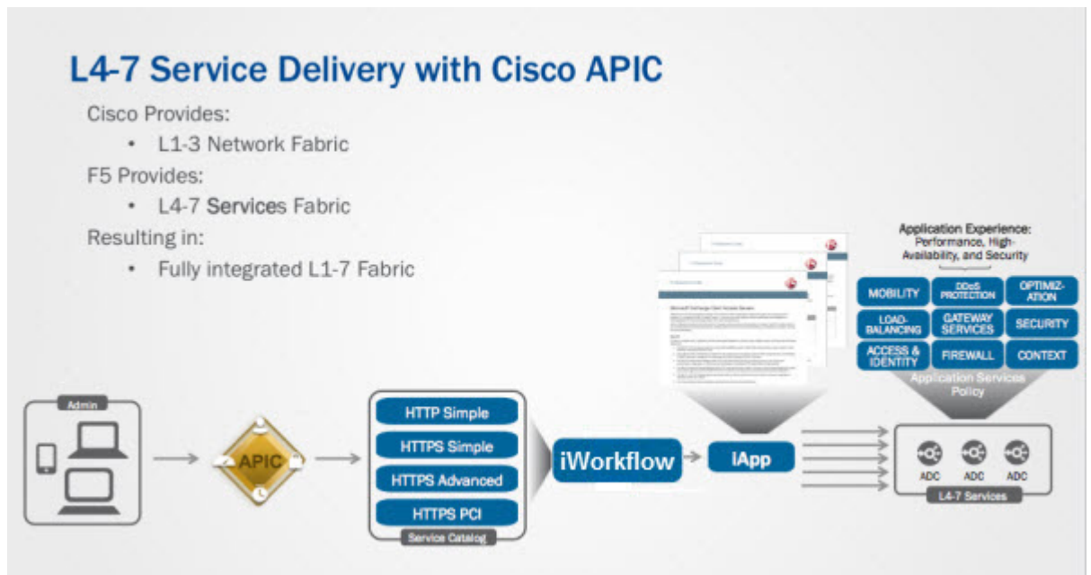
Figure 1: The logical flow between Cisco APIC and the BIG-IP system
